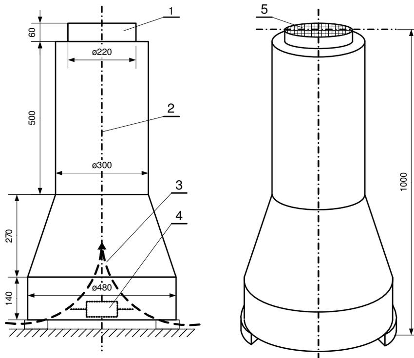
Fig. 2. Scheme of experimental device: 1 – outlet air temperature; 2 – inlet air temperature; 3 – inlet air; 4 – heater with thermostat; 5 – sieve with products
