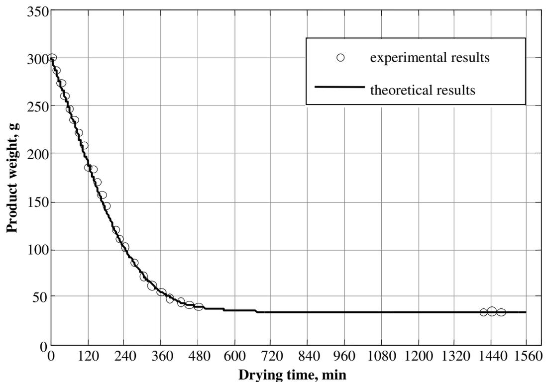
Fig. 3. Carrot slices weight changes during drying process
