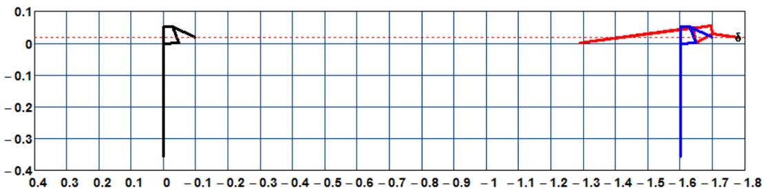
Fig. 6. Positions of virtual manipulator at the initial position and after making a full working cycle (left) and after finishing the returning stroke and turning to the working position (right)
