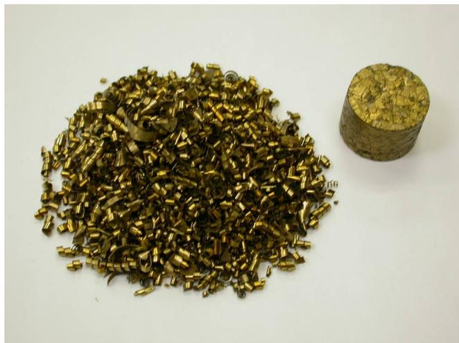
Fig. 1. Chips before and after briquetting
