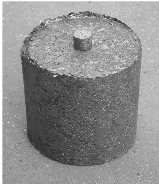
Fig. 2. **Briquettes from steel and brass chips**
