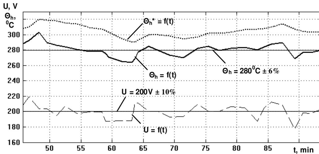
Fig. 7. Simulated characteristics of heater temperature for stationary model ( $\Theta_h^* = f(t)$ ) and for non-stationary self-tuning up model ( $\Theta_h = f(t)$ ) under random variable voltage ( $U = 200\text{V} \pm 10\%$ )
