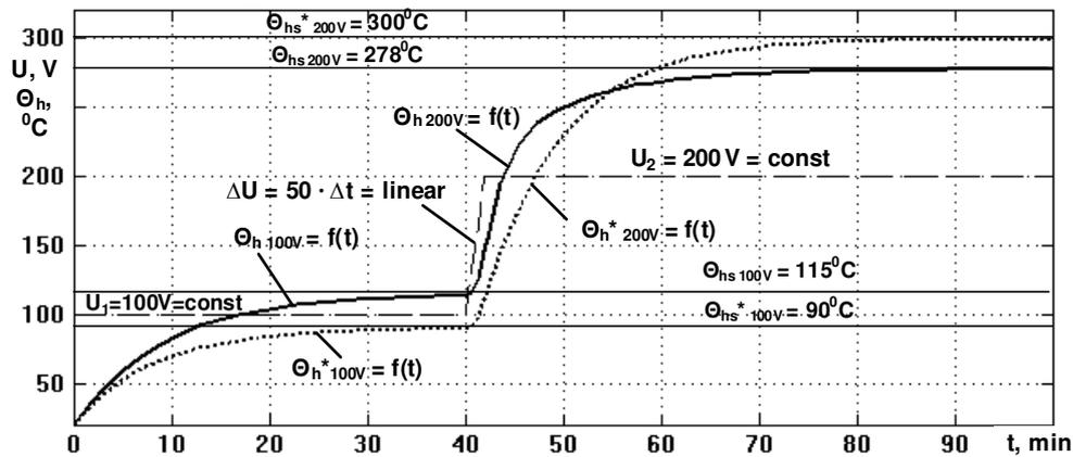
Fig. 4. Simulated characteristics of heater temperature for stationary model ( $\Theta_h^* = f(t)$ ) and for non-stationary self-tuning up model ( $\Theta_h = f(t)$ ) under step and linear growing voltage ( $U_1 = 100 \text{ V}$ ,  $\Delta U = 50 \cdot \Delta t$ ,  $U_2 = 200 \text{ V}$ )
