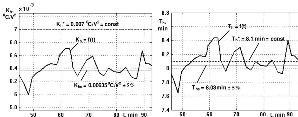
Fig. 6. Characteristics of sensitivity and inertia factors for stationary model ( $K_h^* = 7 \cdot 10^{-3} \text{ }^\circ\text{C} \cdot \text{V}^{-2} = \text{const}$  and  $T_h^* = 8.1 \text{ min} = \text{const}$ ) and for non-stationary self-tuning up model ( $K_h = f(t)$ , and  $T_h = f(t)$ ) under random variable voltage ( $U = 200 \text{ V} \pm 10\%$ )
