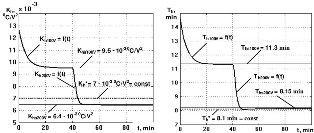
Fig. 3. Characteristics of sensitivity and inertia factors for stationary model ( $K_h^* = 7 \cdot 10^{-3} \text{ } ^\circ\text{C} \cdot \text{V}^{-2} = \text{const}$  and  $T_h^* = 8.1 \text{ min} = \text{const}$ ) and for non-stationary self-tuning up model ( $K_{h \ 100 \text{ V}} = f(t)$ ,  $K_{h \ 200 \text{ V}} = f(t)$  and  $T_{h \ 100 \text{ V}} = f(t)$ ,  $T_{h \ 200 \text{ V}} = f(t)$ ) under two step voltage ( $U_1 = 100$  V,  $U_2 = 200$  V)
