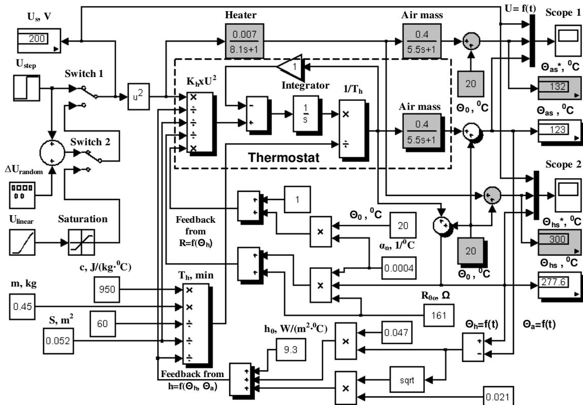
**Fig. 2. Block diagram for transient process simulation of stationary and non-stationary electrical heater models with calculation of variable sensitivity and inertia factors during simulation**
