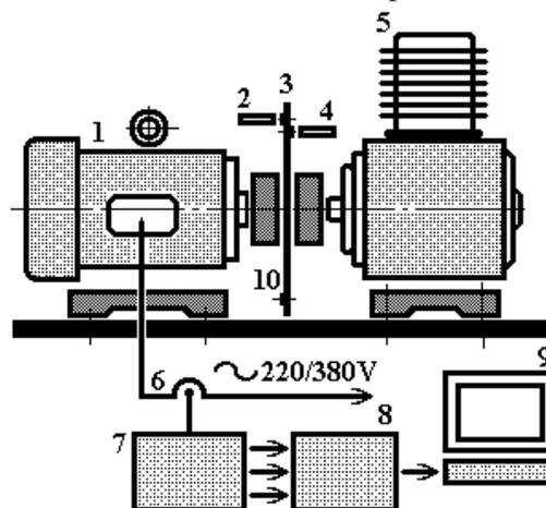
Fig. 6. The scheme of experimental installation for the monitoring of bearing units of electric motor:
