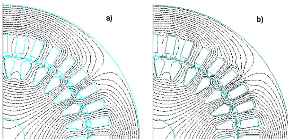
Fig. 2. Calculation of magnetic field of induction motor (pole distribution –  $\tau$ ):
