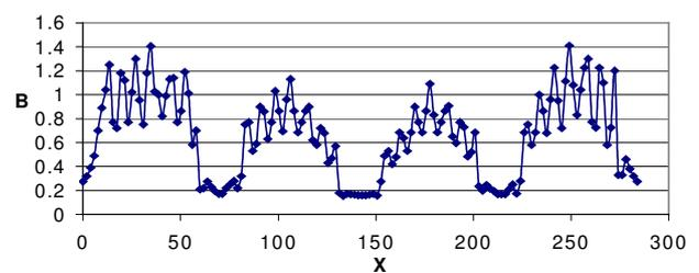
Fig. 4. Induction distribution in the motor air gap without the faults
