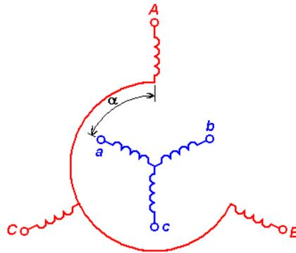
Fig. 1. Model of the induction motor windings
