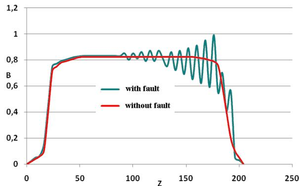
Fig. 5. Induction distribution in air gap along the axis direction of the motor with and without fault in the bearing unit
