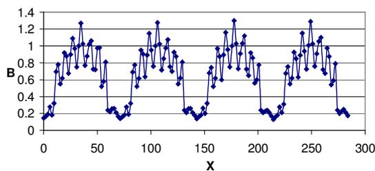
Fig. 3. Induction distribution in the motor air gap with the faults
