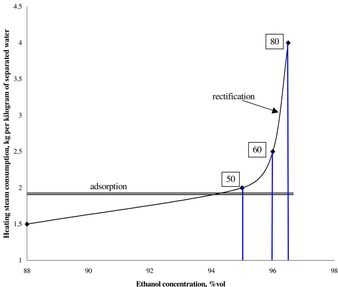
Fig. 2. Energy consumption in rectification and water adsorption processes:
