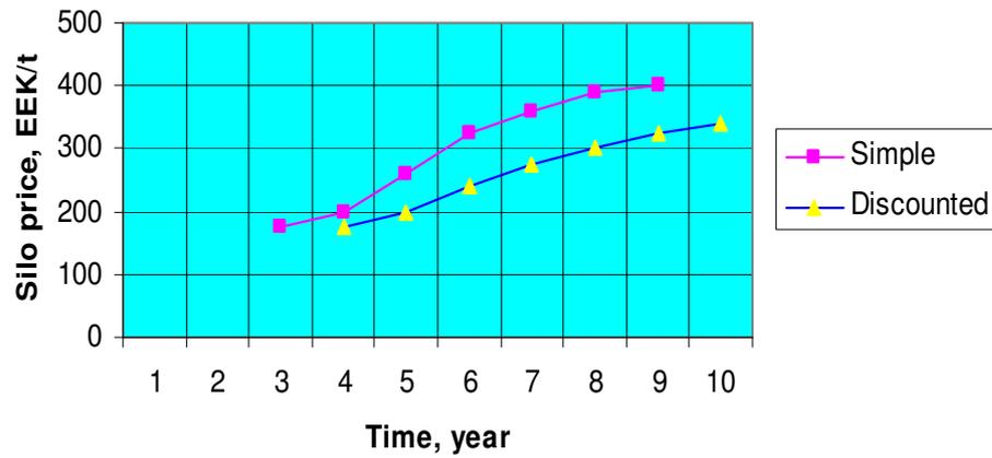
Fig. 1. Simple and discounted payback time depending on the silo price (electric sales tariff 1.25 EEK kWh<sup>-1</sup>)
