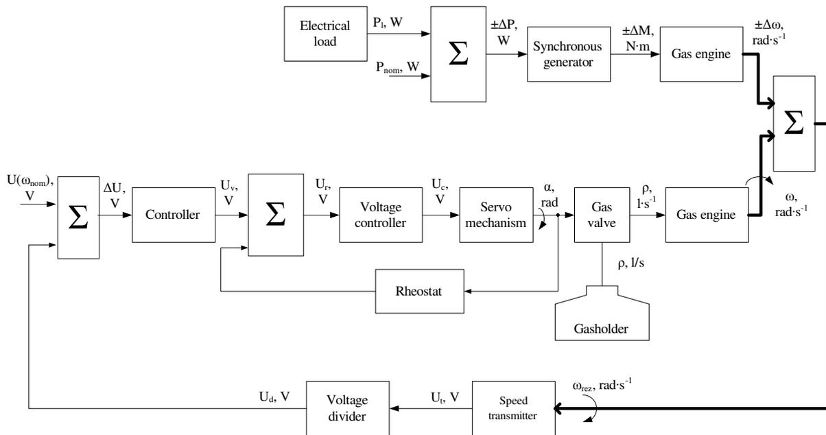
Fig. 1. Block diagram of cogeneration plant automatic control system
