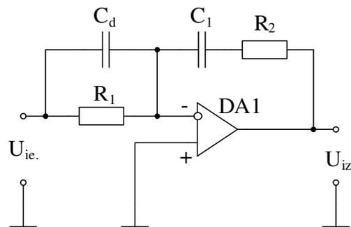
Fig. 3. Electrical diagram of PID controller
