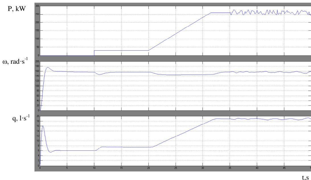
Fig. 4. **Transient curves of cogeneration plant:**  $P$  – electric load,  $\omega$  – rotation frequency,  $q$  – consumption of biogas
