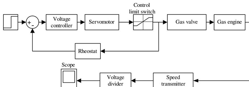
Fig. 2. Block diagram for determination of the controller type and tuning parameters
