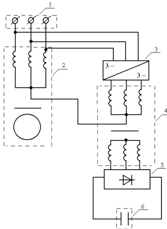
Fig.1. Induction drive with stator side energy storage system
