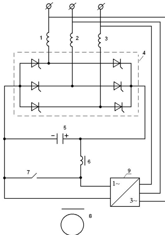
Fig. 2. Induction drive with parametric pulse converter and energy storage system
