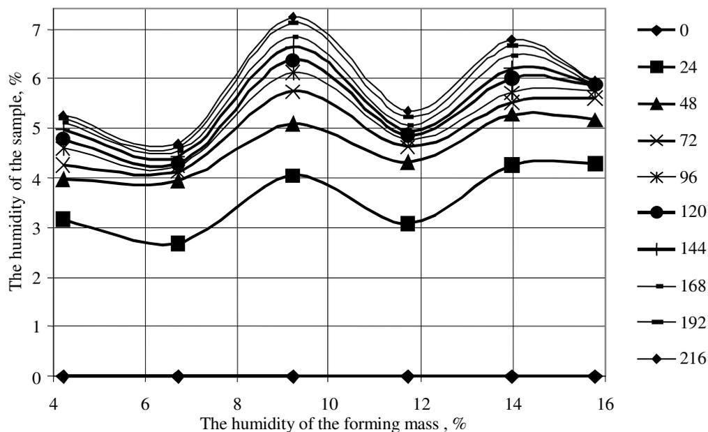
Fig. 4. Dependence of sample humidity on humidity of the forming mass at various duration of samples' storage above water. Numbers at the curves are sample's storage duration in hours
