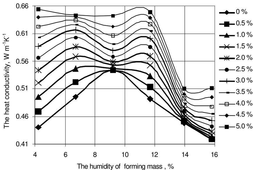
Fig. 3. Dependence of heat conductivity on humidity of forming mass with various absolute humidity of samples during investigation
