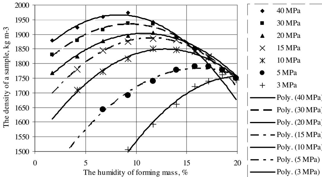
Fig. 2. Density dependence of dried samples on the humidity of forming mass at various extruding pressure
