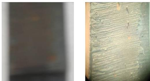
Fig. 1. Plasma cut surfaces of steel 65Mn4 (left) and C80U
