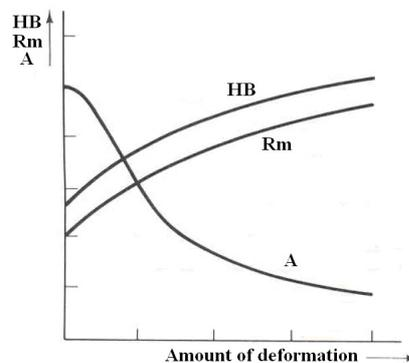
Fig. 3. Influence of deformations on mechanical properties of materials
