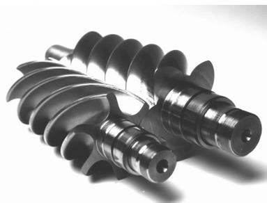
Fig. 1. Rotors of screw type compressor
