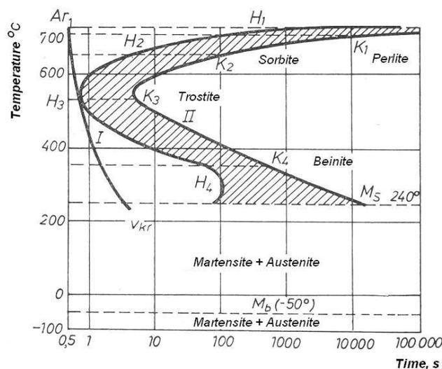
Fig. 6. Curve of austenite isothermal transformation
