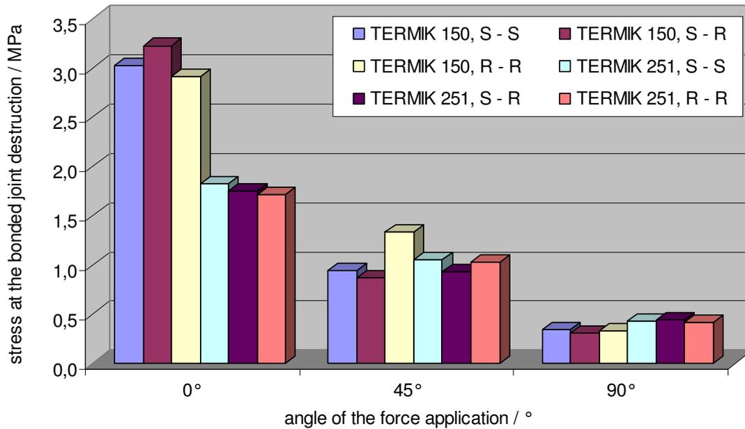
Fig. 3. Test results of the specimens from spruce wood
