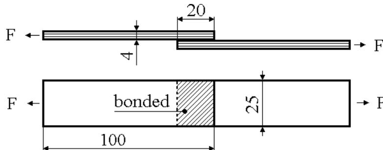
Fig. 1. Test specimens shape and dimensions
