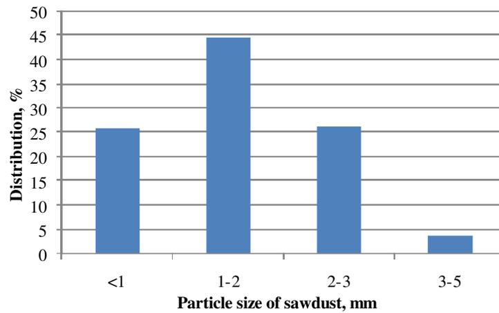
Fig.3. Distribution of particle size of sawdust
