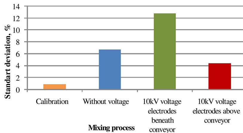
Fig. 8. Quality of mixture in dependence of mixing process
