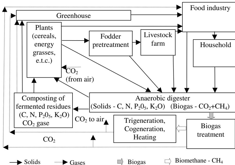
Fig. 1. Scheme of raw materials supply to anaerobic digester and plant nutrients cycling in rural area
