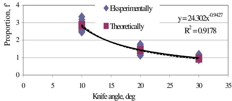
Fig. 6. Generalized coefficient of friction  $f'$
