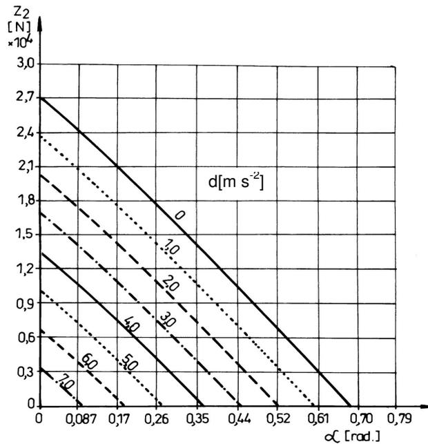
Fig. 4. Variation of loads  $Z_2$  on the tractor rear axle during downhill braking in dependence on the slope angle  $\alpha$ , for various braking decelerations  $d$
