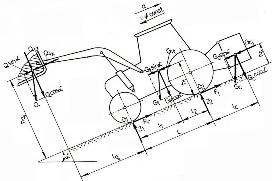
Fig.1. Exterior forces acting upon the tractor-front loader system during downhill braking
