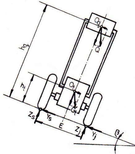
Fig. 3. Forces acting on the tractor - loader system when moving on a transversally slope
