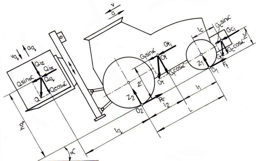
Fig. 2. External forces acting upon the on the forklift truck during braking on a longitudinal descending slope
