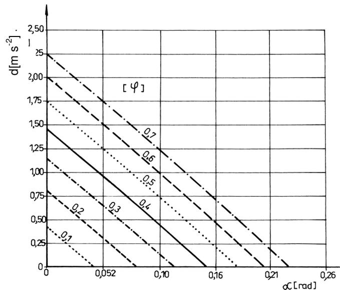
Fig. 5. Variation of the maximum braking deceleration  $d_{max}$  achievable by the 2WD tractor U 650 M depending on the slope tilt angle and various adherence coefficients of the road  $\varphi$
