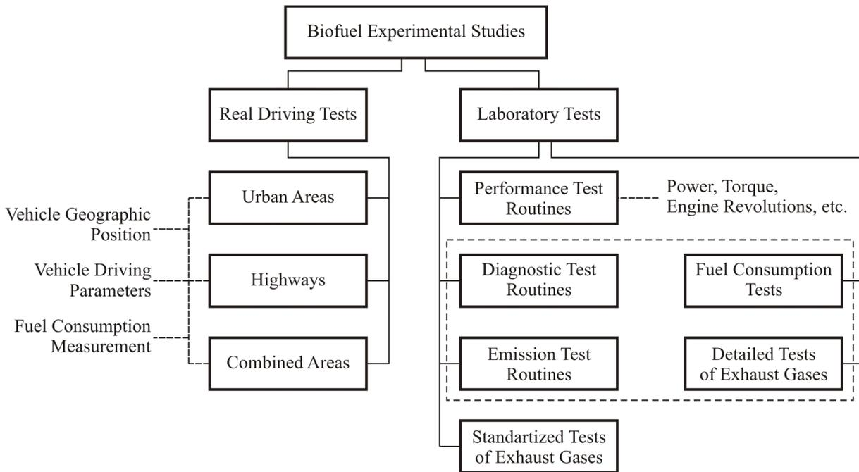
Fig. 1. Flow chart of the procedure for automobile testing
