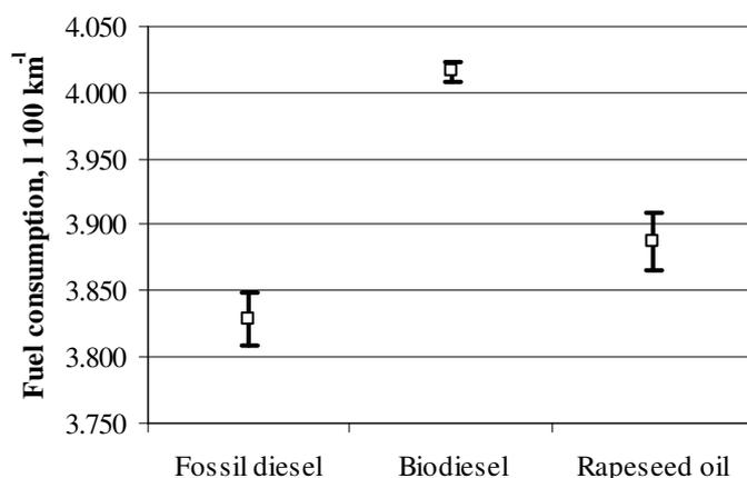
**Fig. 7. Results of pilot test at constant speed (50 km h<sup>-1</sup>) using three different fuels**
