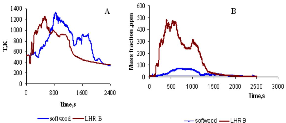
Fig. 2. Time dependence variations of the burning zone temperature (A) and the formation of NO<sub>x</sub> (B) emissions during the burnout of LHR and commercial softwood granules
