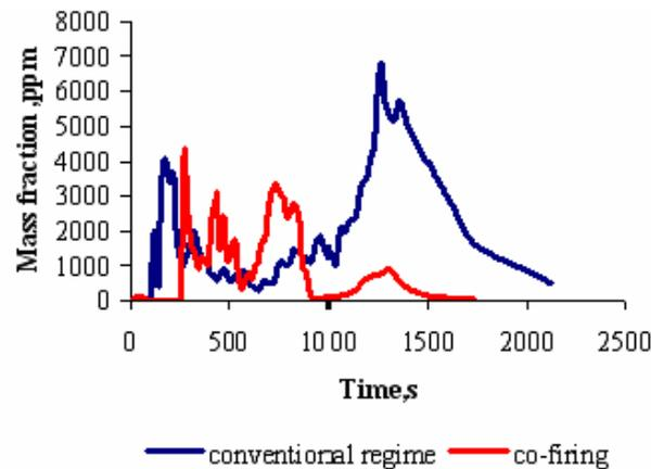
Fig. 3. Time dependence variations of CO emission during the burnout LHR B granules for the self-sustaining and co-firing regimes
