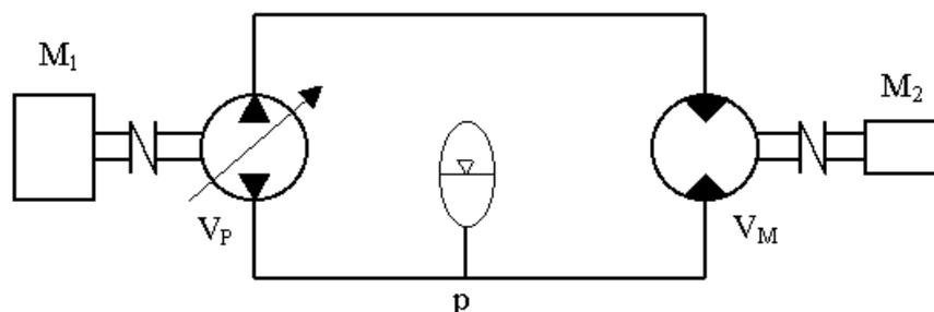
Fig. 1. Hydrostatic transmission scheme of self-moving machines
