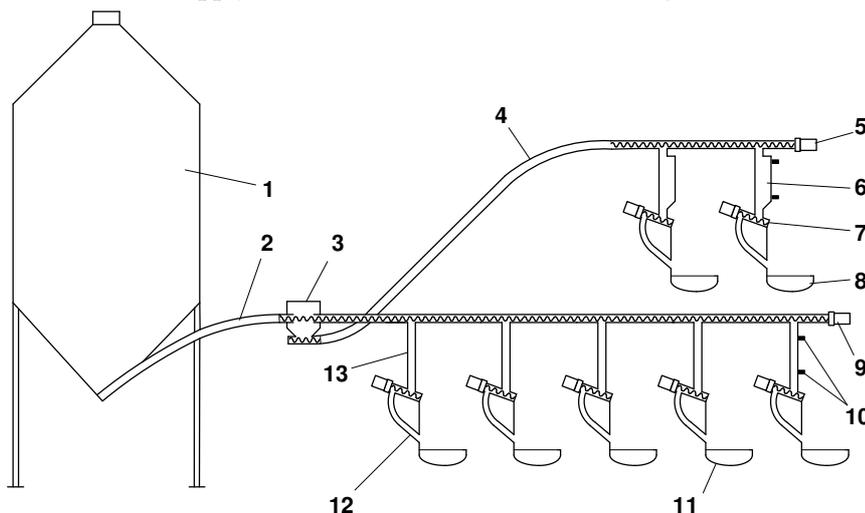
Fig. 1. **Technological scheme of feed concentrate distribution:** 1 - feed concentrate tank; 2 – main coil conveyor; 3 – feed flow distributor; 4 – additional coil conveyor; 5, 9 – electro motor with reducer for driving conveyors; 6 – dosimeter tank; 7 – dosimeter; 8 – milking robot feed troughs; 10 - feed concentrate level sensors; 11 - feed concentrate feeding station; 12 - feed concentrate passage way; 13 - feed concentrate accumulation pipe
