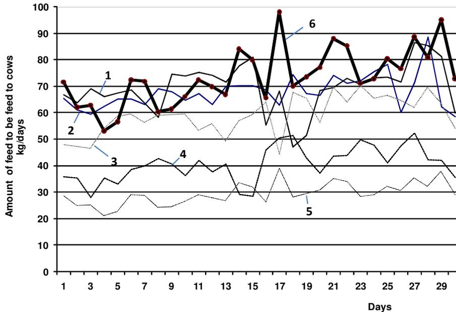
Fig. 4. **Actually supplied and shown by the computer amount of feed concentrate at feeding stations:** 1, 2, 3, 4, 5 – rationed amount of feed correspondingly at the first, second, third, fourth and fifth stations, 6 – actually possible amount of rationed feed
