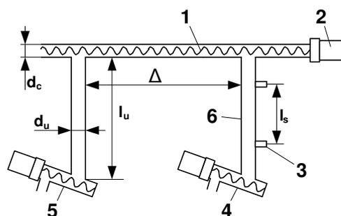
Fig. 2. **Feed concentrate supply line calculation scheme:** 1 – coil conveyor; 2 – drive electro motor with reducer; 3 – feed level sensor; 4, 5 – feed concentrate dosimeters; 6 – feed accumulation pipe
