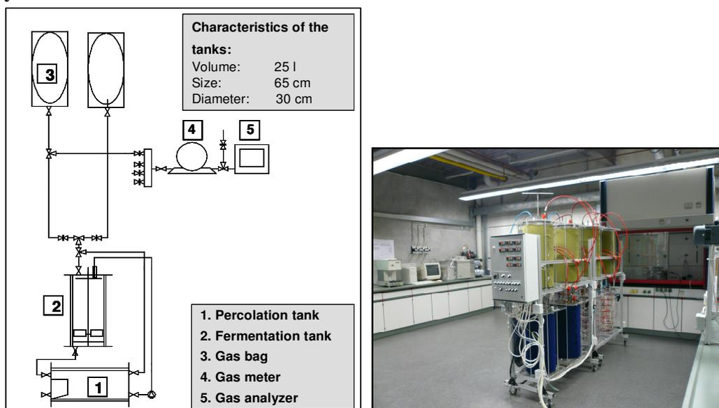
Fig. 1. Test plant for dry fermentation experiments with percolation
