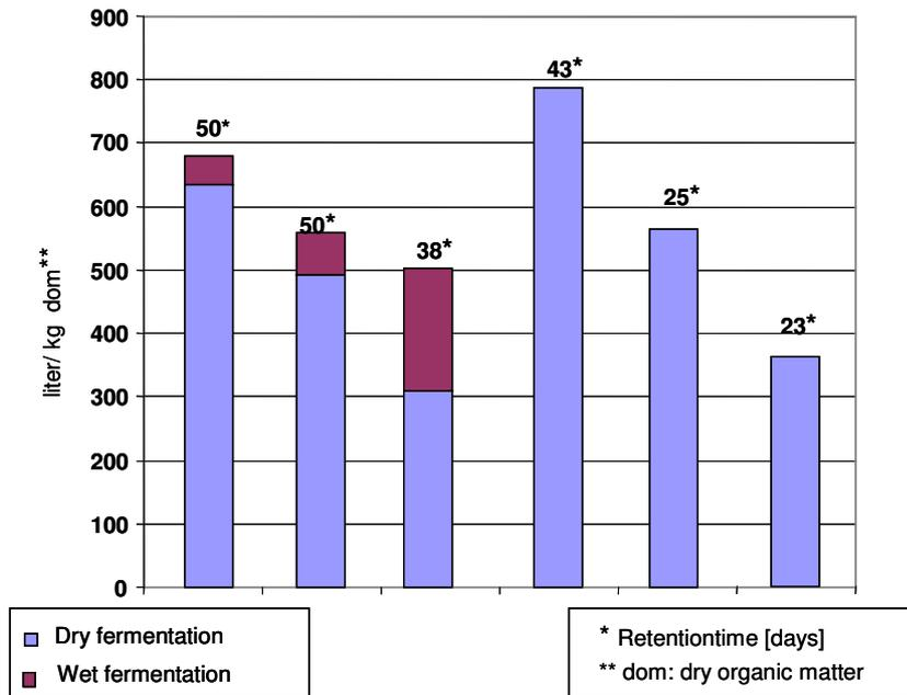
Fig. 3. Biogas yield of the laboratory experiments: dry-wet fermentation compared with dry fermentation
