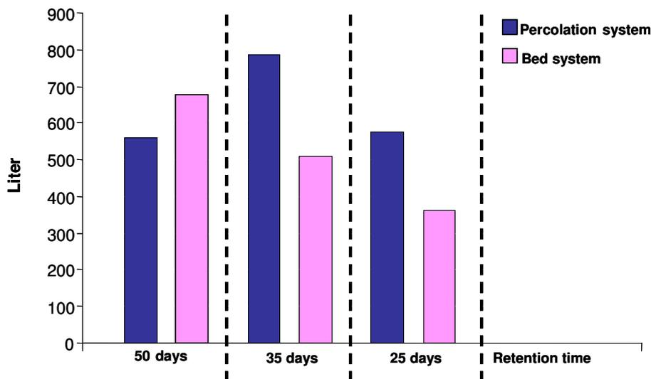
Fig. 5. Biogas yield of the percolation system and the bed system at variable retention time
