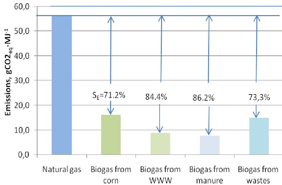
Fig. 3. Emissions and emission savings from biomass usage for biogas production and for heat and power cogeneration
