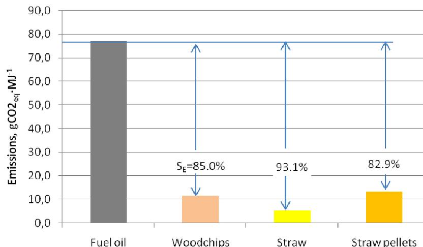
Fig. 2. Emissions and emission savings from solid biomass usage for heat energy production
