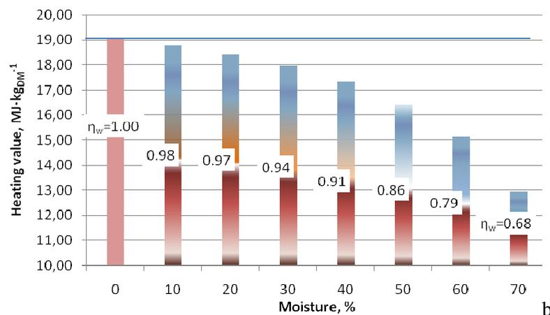
Fig. 1. Heating value of wood biomass per 1 kg dry matter and coefficient  $\eta_w$  for correction of heating value in dependence on biomass moisture
