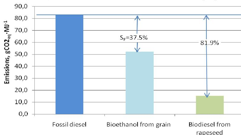
Fig. 4. Emissions and emission savings from bioethanol and biodiesel production and utilisation
