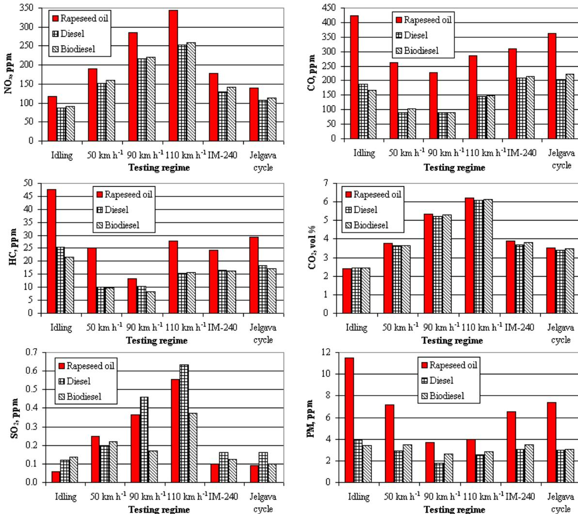
Fig. 9. Exhaust gas measurement results
