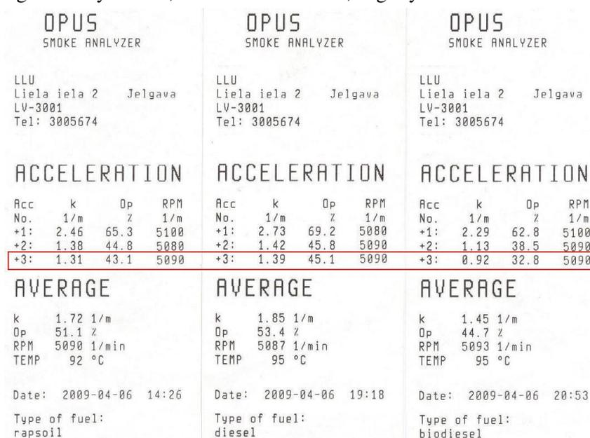
Fig. 8. Absorption coefficient comparison performing smoke analyses
