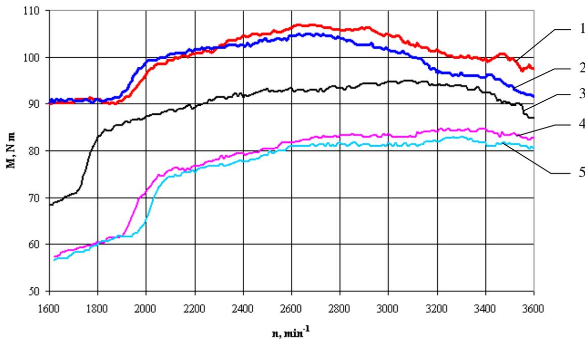
Fig. 6. Torque characteristics operating automobile on three different fuels: 1 – diesel before modifying; 2 – biodiesel before modifying; 3 – rapeseed oil after modifying; 4 – diesel after modifying; 5 – biodiesel after modifying
