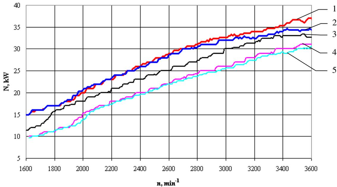
Fig. 5. Power characteristics operating automobile on three different fuels: 1 – diesel before modifying; 2 – biodiesel before modifying; 3 – rapeseed oil after modifying; 4 – diesel after modifying; 5 – biodiesel after modifying
