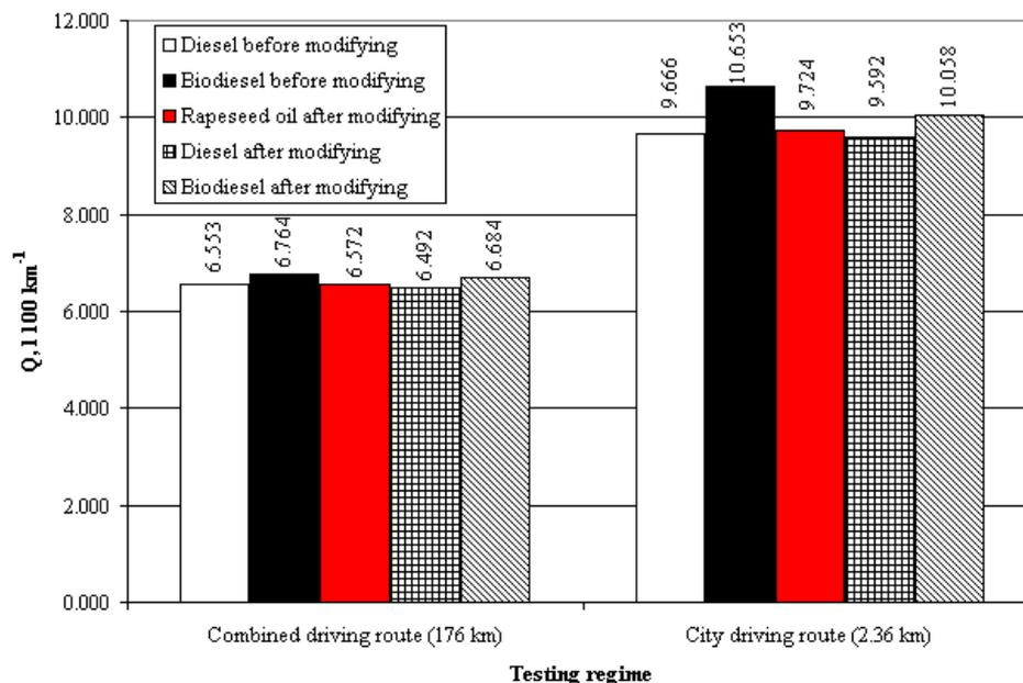
Fig. 4. Fuel consumption comparison performing real driving tests
