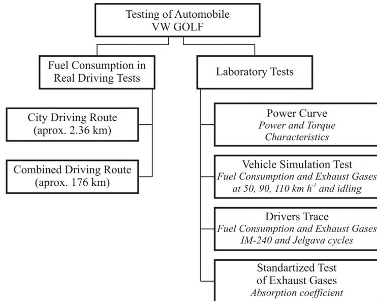
Fig. 2. Flow chart of the procedure for automobile testing
