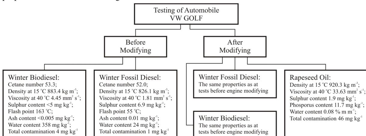
**Fig. 1. Used fuels in testing before and after modifying the engine**
