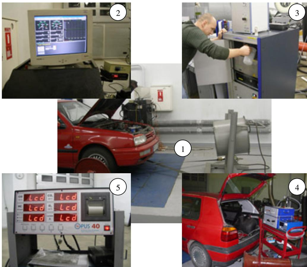
Fig. 3. Laboratory equipment used in automobile testing: 1 – Laboratory Chassis Dynamometer Mustang MD-1750; 2 – Control Platform MDSP-7000; 3 – AVL SESAM FTIR Multicomponent Exhaust Gas Measurement System; 4 – AVL KMA Mobile Fuel Consumption Meter; 5 – OPUS 40 Gas Analyzer
