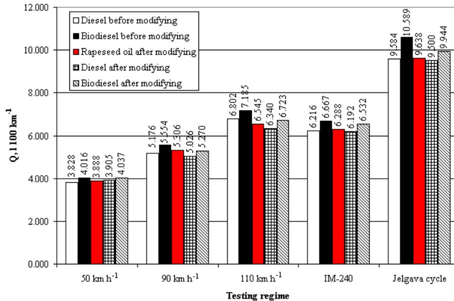
Fig. 7. Fuel consumption comparison performing vehicle simulation test and drivers trace
