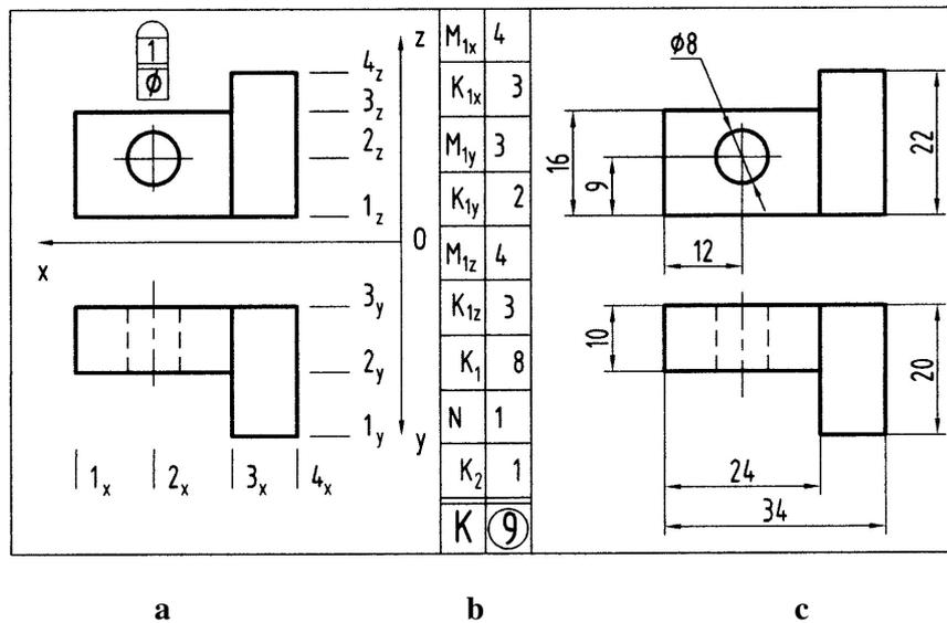
Fig. 3. The number of dimensions for a spatial non-symmetrical part
