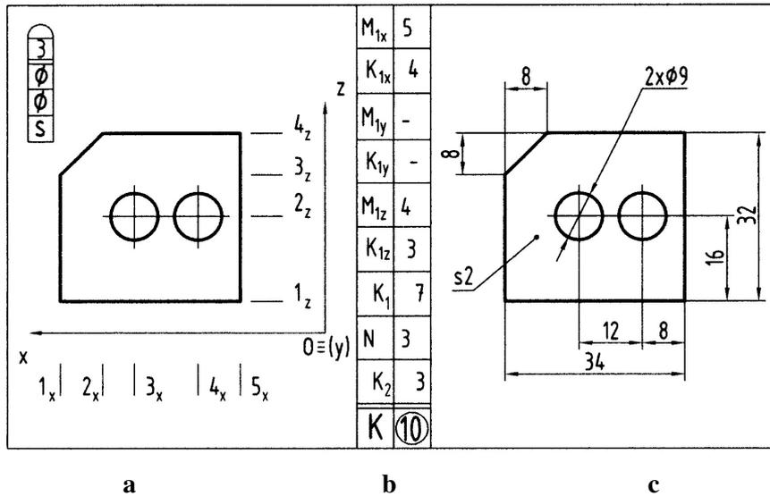
Fig. 4. The number of dimensions for a flat non-symmetrical part
