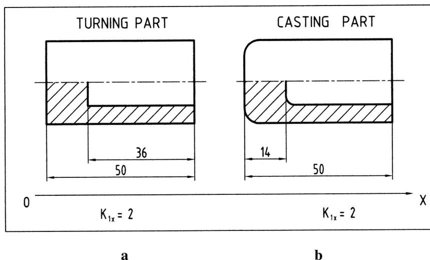
Fig. 2. The number of dimensions for turning part and for casting part
