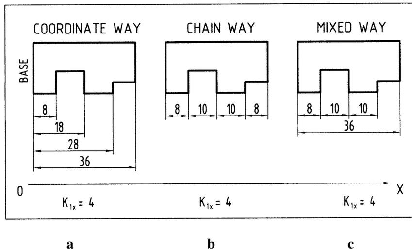
Fig.1. The number of dimensions for plane part according to the ways of dimensions placing
