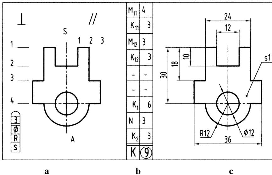
Fig. 5. The number of dimensions for a flat symmetrical part
