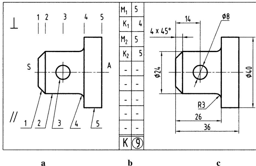
Fig. 6. The number of dimensions for a symmetrical cylindrical part
