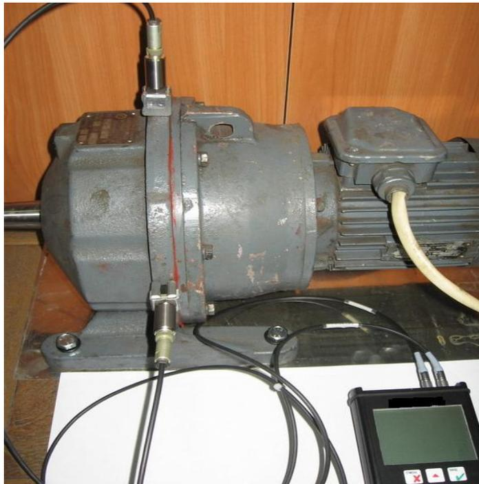
Fig. 1. Planetary reduction gearmotor
