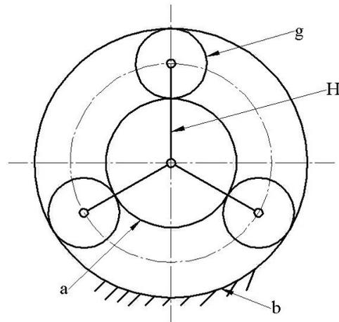
Fig. 2. The scheme of the simplest planetary gearing:
