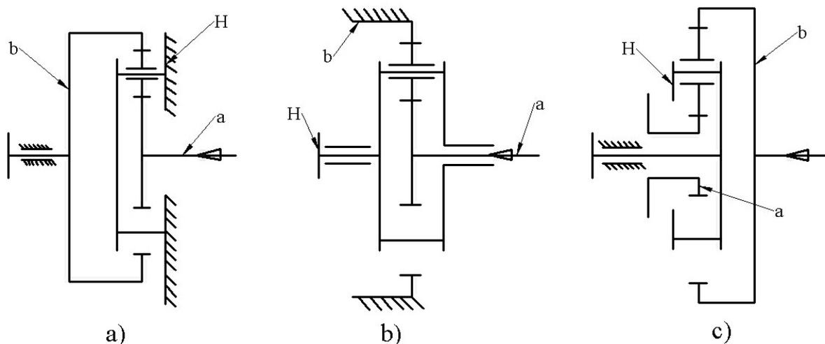
Fig. 3. Kinematics of planetary reduction gearboxes on the basis of one stage planetary gearing:
