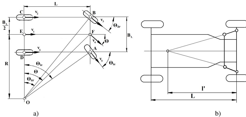
Fig. 1. Turning scheme for an automobile with indeformable wheels (a) and determination of steering parameters (b)
