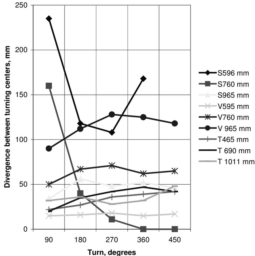
Fig. 3. Divergence between model's turning centres
