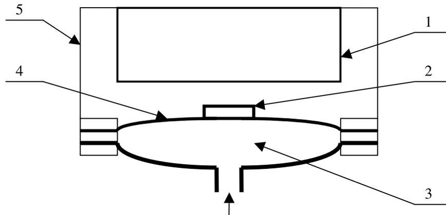
Fig. 4. **Principal scheme of load sensor for pneumatic chamber suspension:** 1 – front magnifier; 2 – micro tenso-resistors; 3 – pressure chamber; 4 – membrane; 5 – casing of sensor
