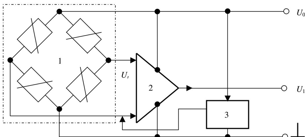
Fig. 5. **Principal circuit of pressure load sensor:** 1 – block of micro tenso-resistors; 2 – converter of signal; 3 – temperature compensator;  $U_0$  – feeding voltage;  $U_1$  – output digital signal;  $U_t$  – output analog signal
