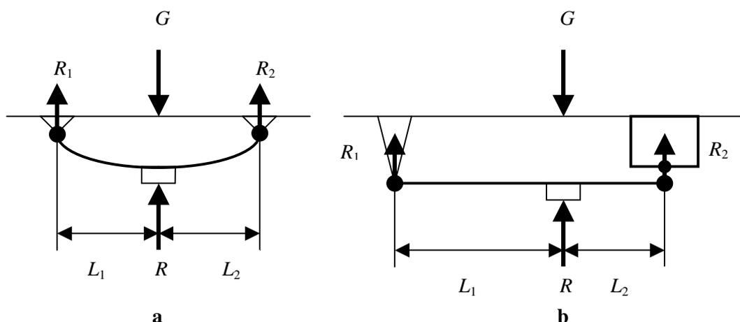
Fig. 1. **Types of suspensions:** a – leaf-type springs; b – pneumatic chamber
