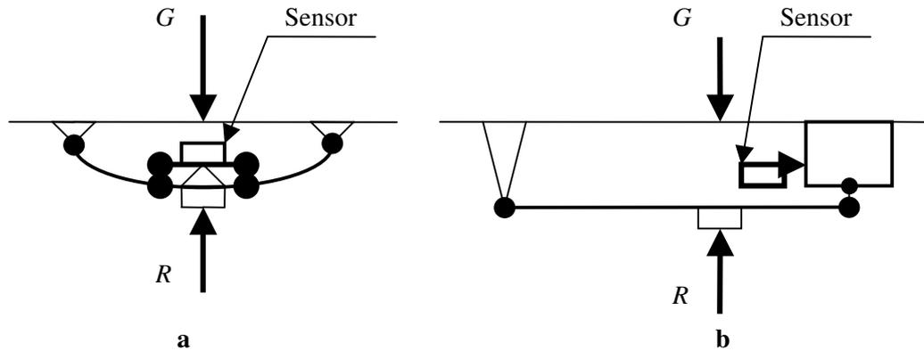
Fig. 2. **Scheme of mounting of load sensors:** a – on suspension of leaf-type springs; b – on suspension of pneumatic chamber
