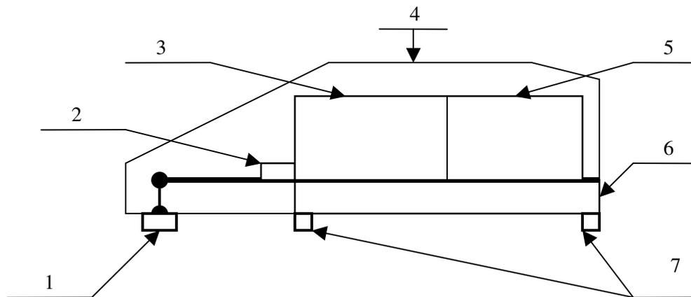
Fig. 6. **Principal scheme of load sensor for leaf-type spring suspension:** 1 – fastening of flexible dipstick; 2 – micro tenso-resistor; 3 - front magnifier; 4 – coating of sensor; 5 – wireless router; 6 – base of sensor; 7 – fastening places of sensor
