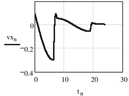
Fig. 3. Velocity  $vx_n$  of mass along x axis in time  $t_n$  domain without hull vibration in SI
