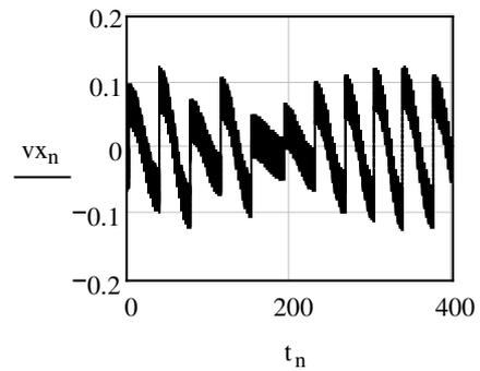
Fig. 5. Velocity  $vx_n$  of mass along x axis in time  $t_n$  domain with hull vibration in SI
