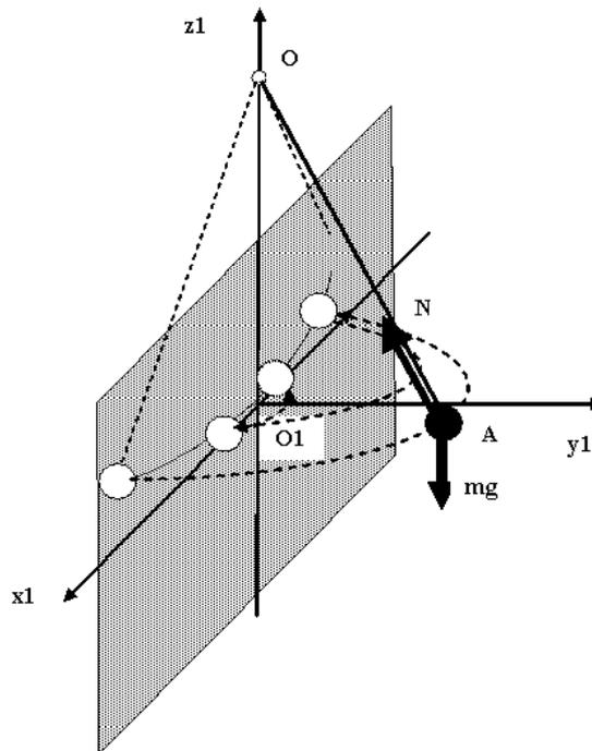
Fig. 1. **Mathematical model of pendulum with one bumper:**  $x_1, y_1, z_1, O_1$  – absolute reference system;  $m$  – mass of pendulum;  $g$  – acceleration of free fall;  $AO$  – length of pendulum;  $H = O_1O - z$  coordinate of pendulum rotation point  $O$ ;  $x_1O_1y_1$  – bumper parallel plane
