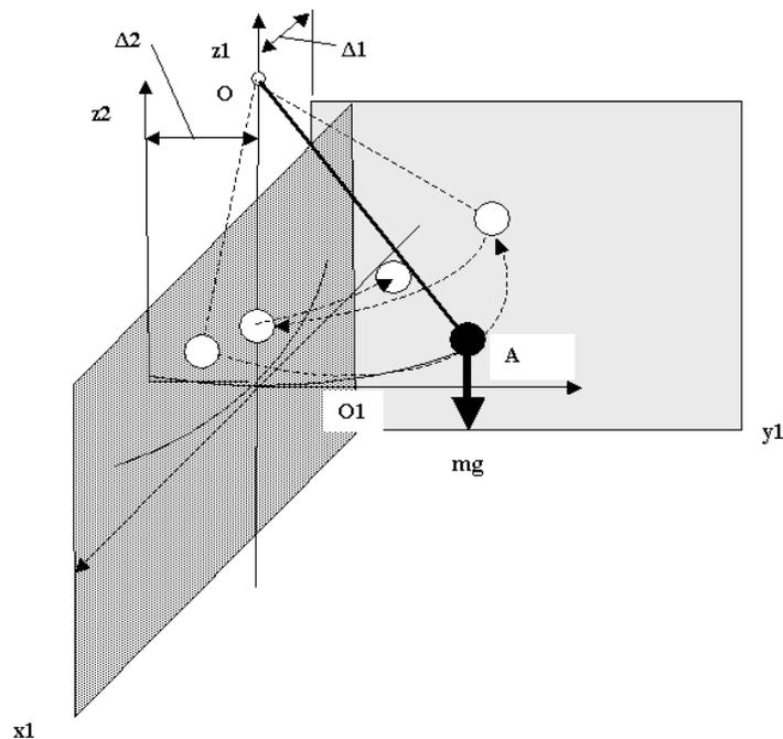
Fig. 6. Mathematical model of pendulum with two bumpers:  $x_1, y_1, z_1, O_1$  – absolute reference system;  $m$  – mass of pendulum;  $g$  – acceleration of free fall;  $AO$  – length of pendulum;  $H = O_1O - z$  coordinate of pendulum rotation point  $O$ ;  $\Delta 1, \Delta 2$  – bumpers gaps
