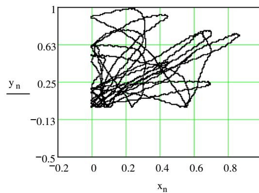
Fig. 10. Motion in plane  $x$ - $y$  with bumpers random vibration in SI
