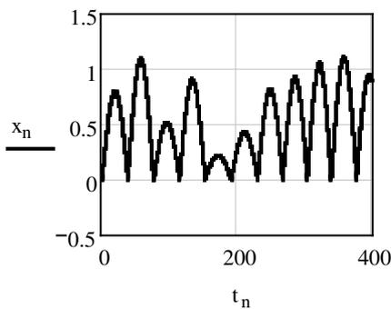
Fig. 4. Displacement  $x_n$  of mass along x axis in time  $t_n$  domain with hull vibration in SI
