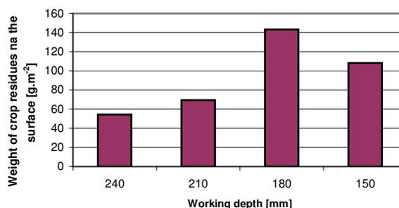
Fig. 6. Weight of crop residues according to working depth
