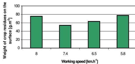
Fig. 7. Weight of crop residues according to working speed
