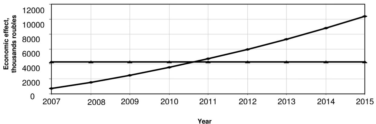
Fig. 5. Graphical calculation of the payback time for the wind turbine use in thousand roubles: —▲— — forecast of total economic effect; —■— —capital investments in the wind turbine construction
