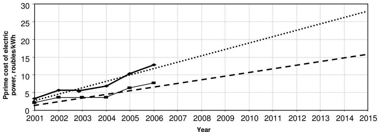
Fig. 3. Growth dynamics of energy prime cost and fuel factor in roubles: —●— — actual growth of energy prime cost; —■— — actual growth of fuel factor; ..... — forecast growth of energy prime cost; — · — forecast growth of fuel factor
