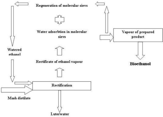
Fig. 1. Flow chart of classical dehydration
