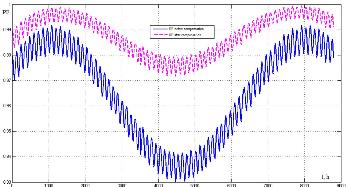
Fig. 3. Reactive electrical power compensation by PasC
