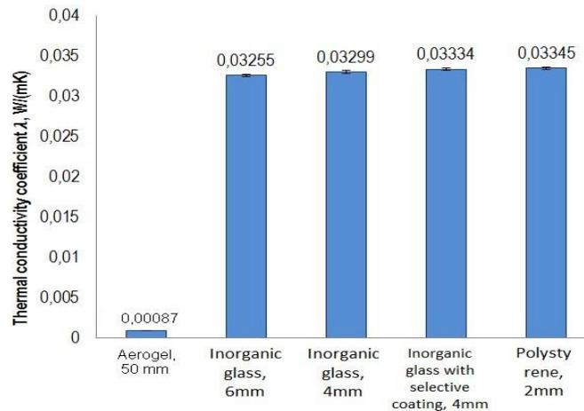
Fig. 3. Values of the thermal conductivity coefficient  $\lambda$  ( $\text{W}\cdot\text{m}^{-1}\cdot\text{K}^{-1}$ ) for each of the materials used in the experiment (average temperature  $T_{\text{average}} = 23$  °C, temperature difference  $\Delta T = 20$  K, sample thickness  $\Delta x = 2$  mm)
