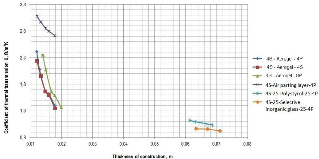
Fig. 10. Dependence of the thermal transmission coefficient  $U$  ( $W \cdot m^{-2} \cdot K^{-1}$ ) on sample thickness
