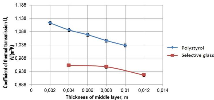
Fig. 9. Thermal transmission coefficient for the samples of organic glass (polystyrene) and inorganic glass with selective coating in the middle layer
